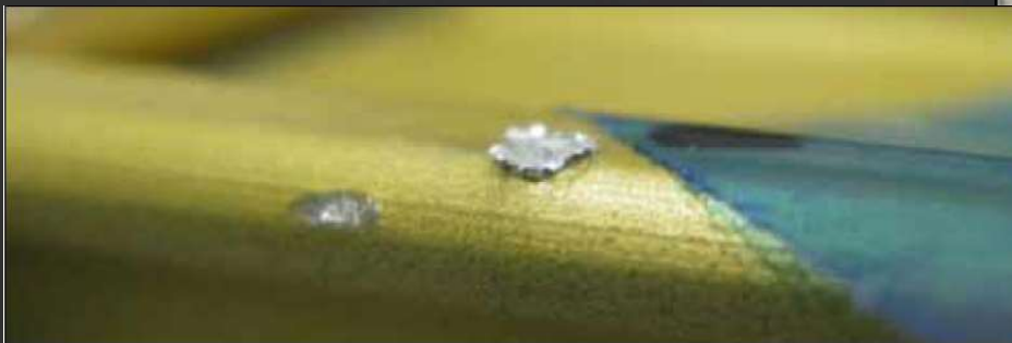
Figure 3. Largest crater found on the PMIA handrail was 1.85 mm diameter with 0.33-mm-high crater lips.
