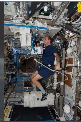
CEVIS (Cycle Ergometer with Vibration Isolation & Stabilization)
